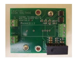
Fig 3.Top View: Adaptor-P5V with V1000-ISO
