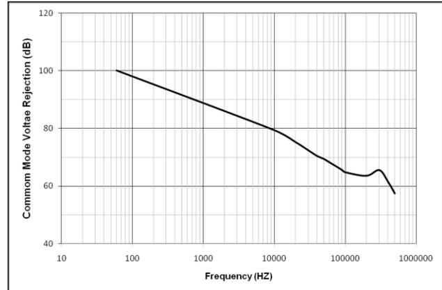
Figure 16: Common Mode Frequency Response
