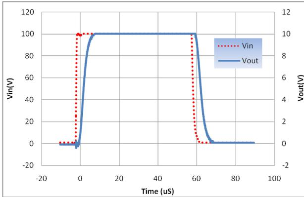
Figure 13: 1000V Input Step Response
